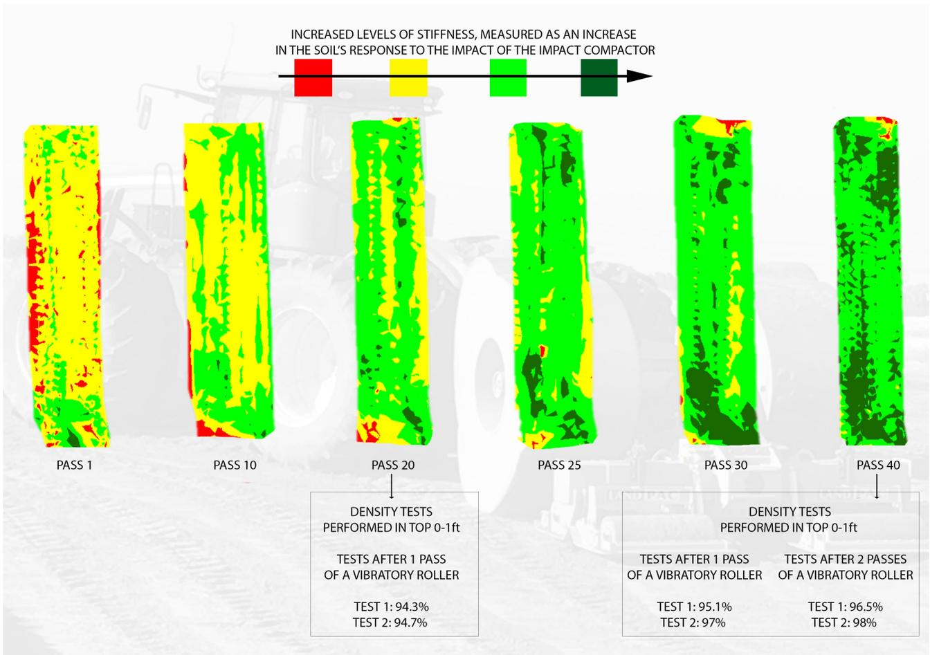
The mapping below shows the final pass only, but in this case a correlation against the minimal density tests performed on site was provided. It basically gives an indication of where the density specification is below 95%, shown in red. Note, however, that with all the maps, the turning circles will be sub-standard due to the reduction in compaction speed and the "dragging" of the roller.
